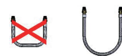
UK: The hose/flexible pipe must have a soft bend
